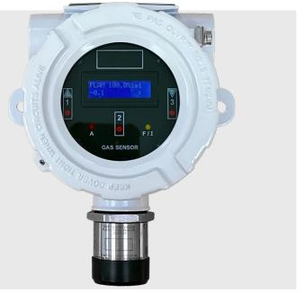
The XDIwin-F1+ Gas Sensor is capable of utilising a wide range of sensor cell types offering an unmatched number of gases that may be monitored. Standard 4~20mA signaling with CANbus address enables the sensors to be networked via the GDS Combi control system or customer preferred monitoring systems. Adjustments to menu settings and readings may be made by a single magnet without the removal of the enclosure lid, alternatively push button adjustment is accessible by removing the lid.
