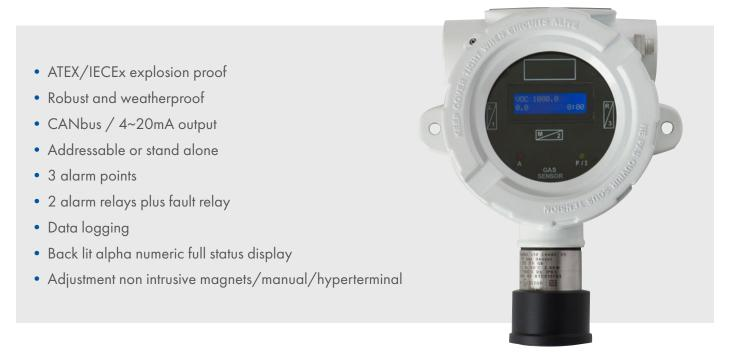
The XDIwin–PID (photoionization detector) is used to measure volatile organic compounds in the low ranges of 0 to 50ppm and 0 to 1000ppm. The unit is fully certified as a flameproof fixed monitor for use in hazardous areas. 4~20mA signaling with CANbus address enables the sensors to be networked via the GDS Combi control system or customer preferred monitoring systems.
